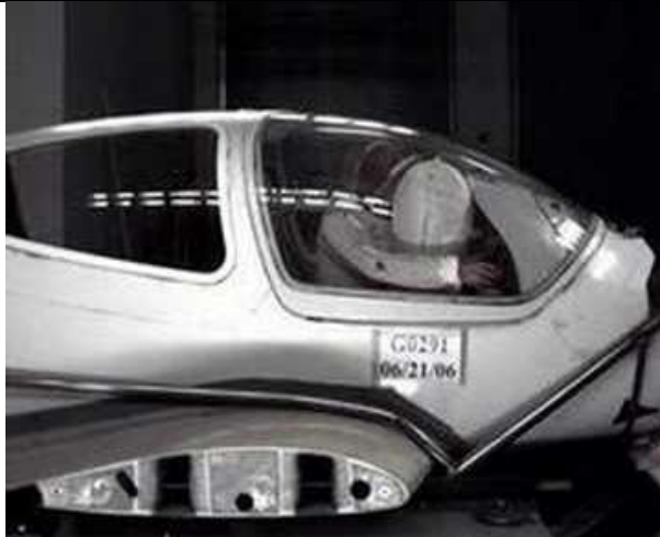
Figure 3. The Mooney airbag and the crash test of the Diamond Da-40 type aeroplane fitted with it [6][7]
