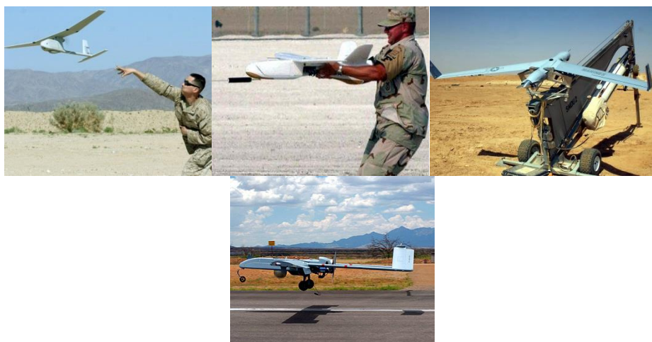
Fig. 1. Launch UAV by hand-drop, bungee, catapult and gear 4 5 6 7
