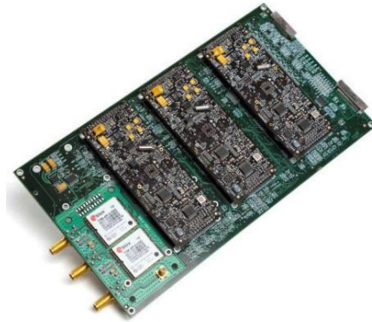
Fig. 2 MP21283X motherboard of three independent autopilots – with voting logics 8
